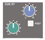
Provides a Stereo Send primarily for Cue purposes. By default the signal is sourced pre fader but additionally it can be sourced after the Channel Fader by selecting "**POST**". It may be worth bearing in mind that if you are using X-Panda in conjunction with an X-Desk and on the X-Desk are using the "**Cue to MIX**" function you may wish to turn this **CUE ST** send off on the X-Panda Stereo channels.
